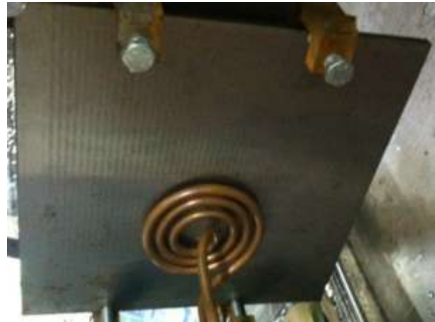
Figure 2. The experiment model for local induction hardening
